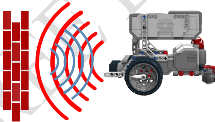
Figure 69 Obstacle detection with ultrasonic sensor
