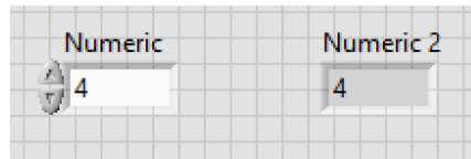
Figure 13 Displays the input number at the output in the Front Panel window
